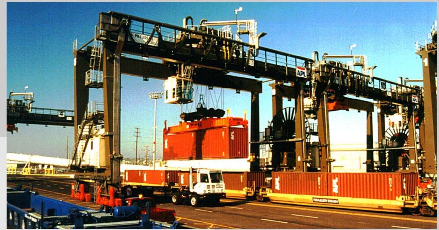
10 RMG cranes for American President Lines (APL) intermodal terminal in sea port of Los Angeles, USA
